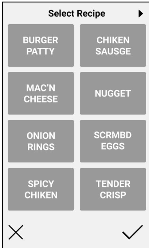
Use the left and right navigation buttons to scroll through the available recipes for this RFHU. To assign a new recipe to the well, simply select the desired recipe.
