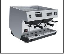
Quick Reference Specifications Dimensions: 23"(H)X 23"(L)X 25"(W) Weight: 122 lbs (full) Electrical Requirements: Volts: 208-240/Watts: 4700/Amps: 30 Plumbing Requirements: Flow: 30GPH (minimum) Pressure: 20psi (minimum) Hardness: 3 GPG (maximum) Fitting: 1/2" NPT Male w/shut off
