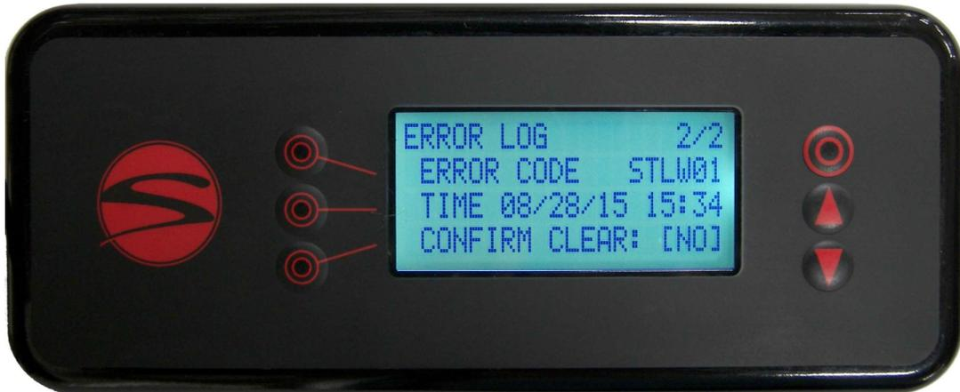
To clear the Error Log, press the 4th line button 2 times so that [CLEAR] is flashing. Press an arrow button to select clear. The 4th line will ask you to confirm clearing the error log as shown below.
