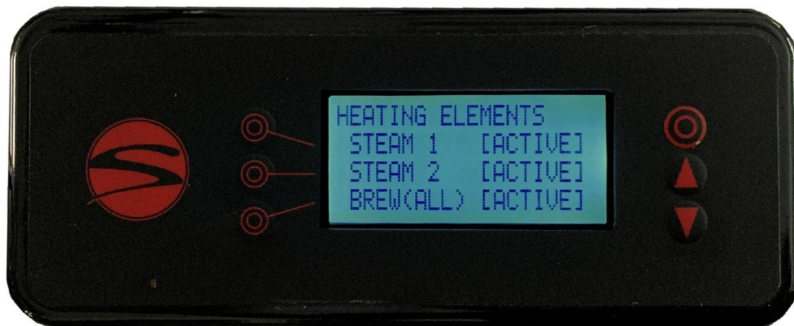
During certain maintenance procedures or technical troubleshooting, it may be necessary to disable sections of the machine's heating system. For proper performance of the machine, all elements should be left active during normal operation.
