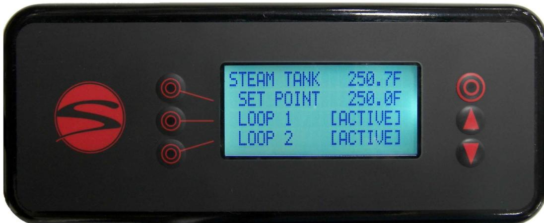
Line 1 shows the current reading of the steam tank temperature probe ("250.7F" in this example). Once this temperature reaches the set point, the digital display will continuously cycle up and down by small increments as the electronics balance the temperature.
