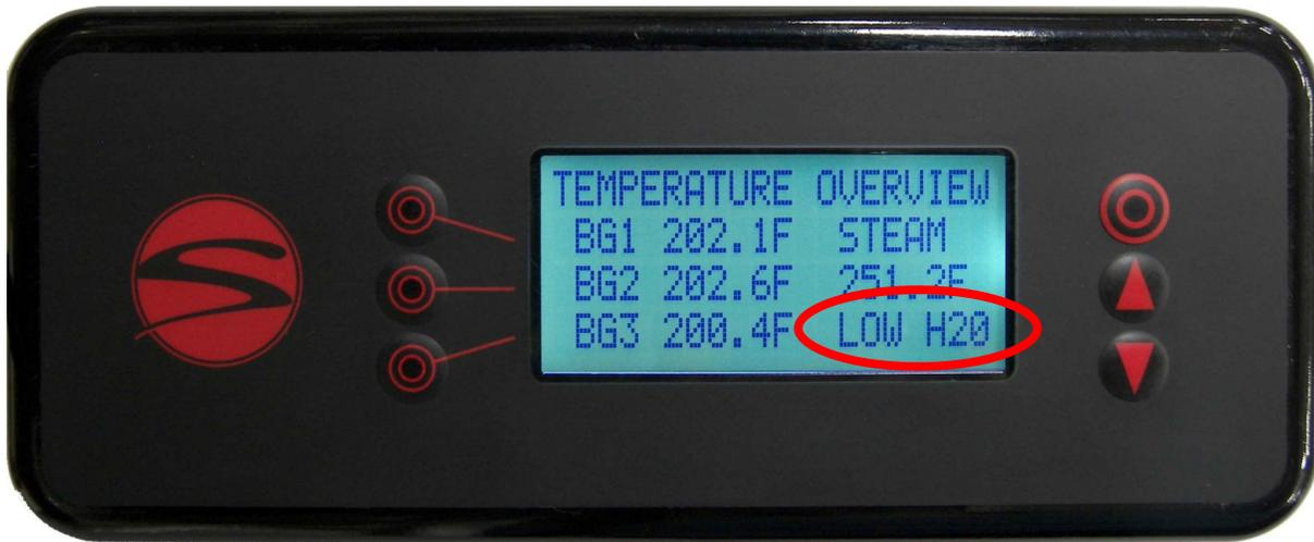
In an effort to prevent damage to machines and to help operators troubleshoot issues, Synesso™ has engineered several safeguards into the programming. By understanding these codes, operators can remedy issues more quickly. The most recent error can be found on the temperature overview screen at the lower right corner.
