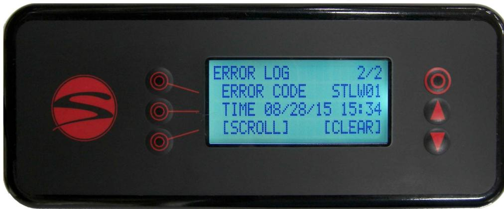
Line 1 of the error log screen shows how many errors the machine has recorded, up to the 35 most recent errors, and which of these you are currently viewing. This example is showing “2/2”, indicating the second of two errors is displayed.
