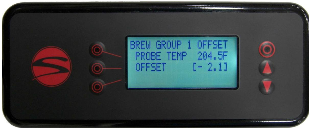
Line 2 indicates the measured water temperature at the selected brew group’s temperature probe.
