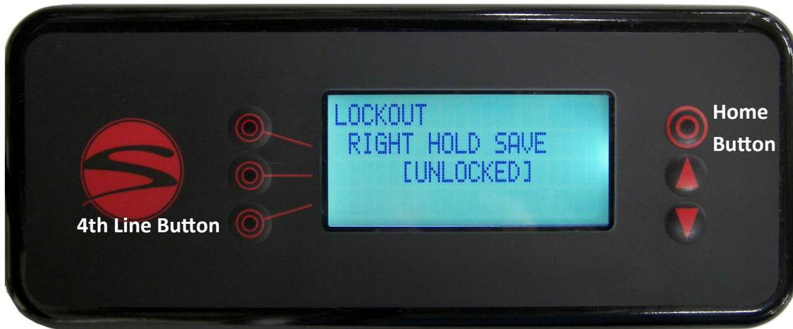
This is the first screen of the 2nd level menu, the save lockout screen.
