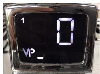
Hold handle LEFT to change the Operation Mode from M (Manual) to MP (Manual Program) to VP (Volumetric Program).
