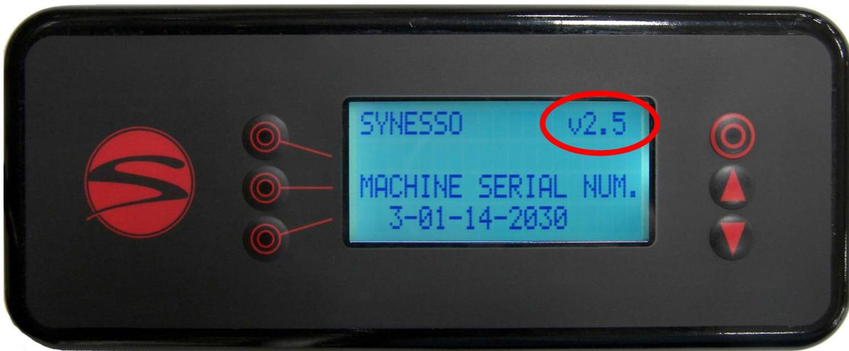
The start-up screen appears momentarily when the machine power is cycled on. The firmware can be viewed in the upper right corner of the screen, in this case v2.5.
