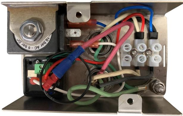
To connect the power cord: Insert the color coded pump cable into the opening of the matching bypass box and attach the wires to the terminal as shown in the picture to the left: green wires stacked on the ground bolt, white matches across to white/red on terminal block, black matches across to black/blue on terminal block, and the male bullet connector on the black wire connects to the female bullet connector on the red wire.
