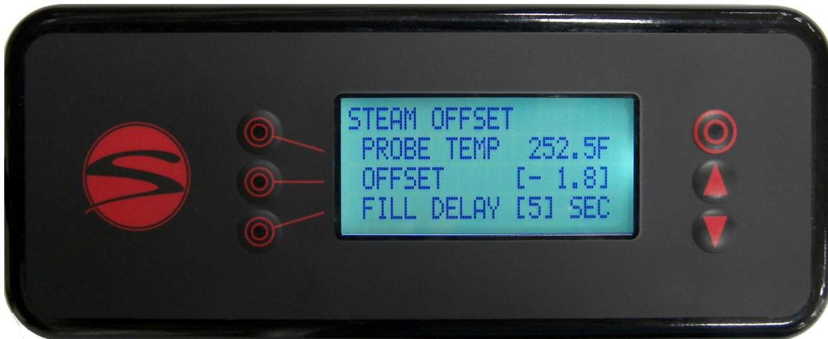
Line 2 indicates the measured steam temperature at the steam tank temperature probe.
