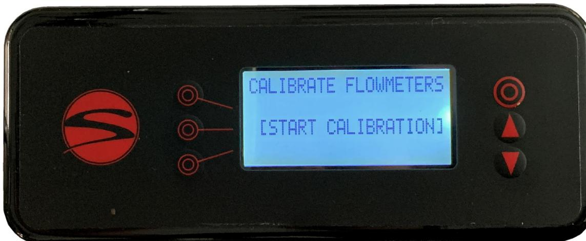
The flowmeter calibration feature is made available with firmware 2.64v.
