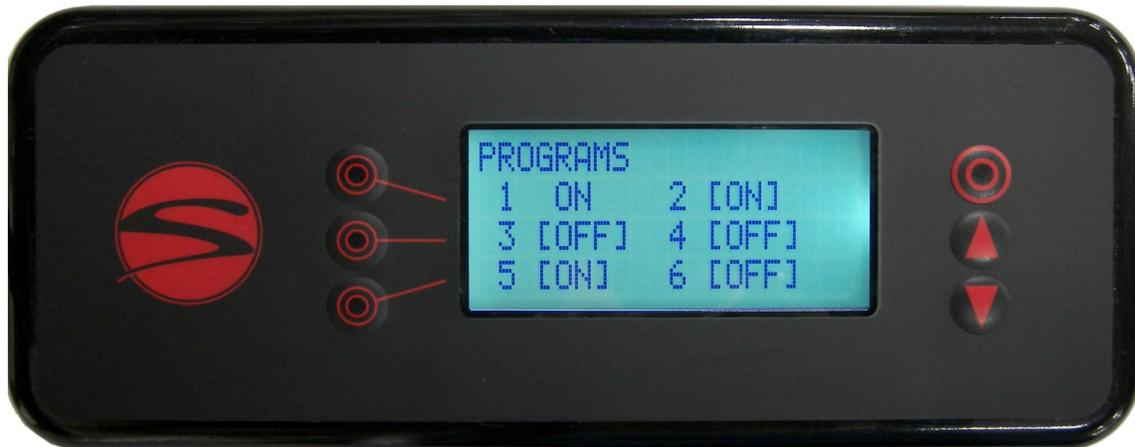
On this screen, you can activate or deactivate program storage positions 2 through 6. Program #1 cannot be deactivated. Shifting right while not brewing a shot will cycle through any program save locations currently active in numerical order. (1->2->5->1... as shown.) This setting is applied to all groups.
