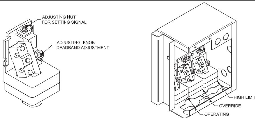
1. Turn the adjusting knob clockwise to the deadband to maximum.
