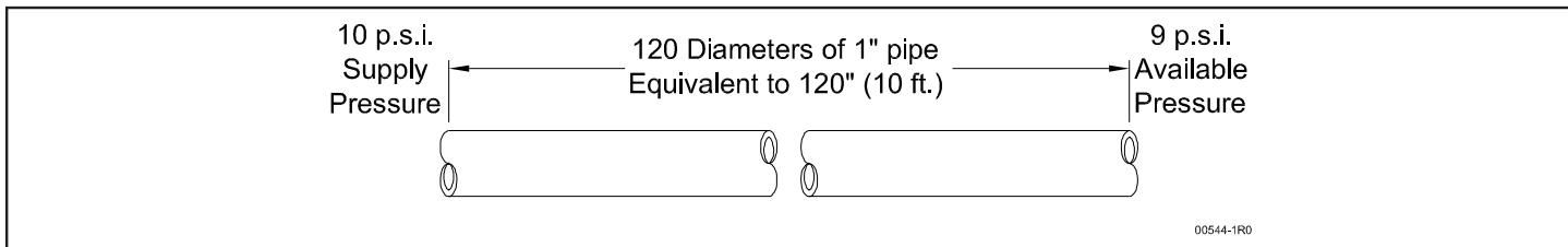
**NOTE:** In 3/4" pipe size, that a Standard 90° Elbow and Angle Valve and a Globe Valve are equivalent to 1.8 feet, 10 feet and 18 feet respectively of straight pipe.
