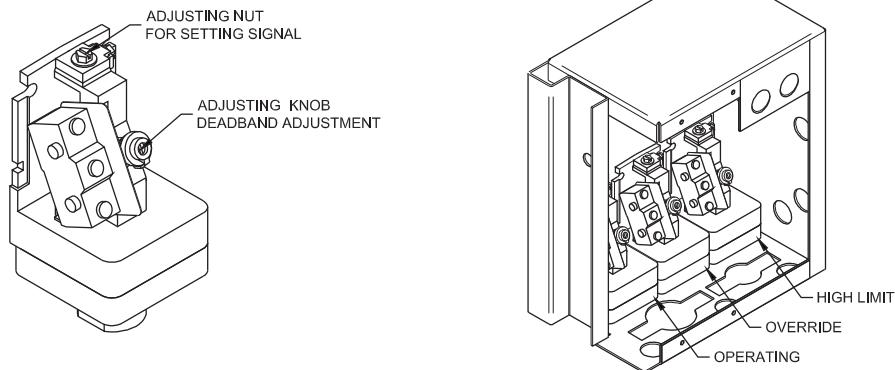
1. Turn the adjusting knob clockwise to the deadband to maximum.
