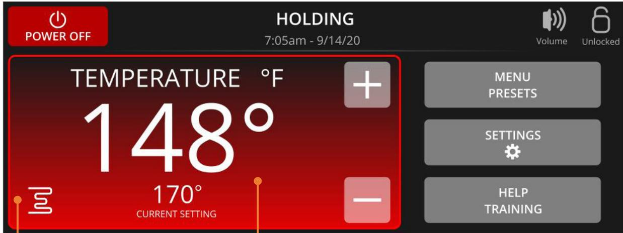
Element Indicators for heat is shown whenever elements are energized
