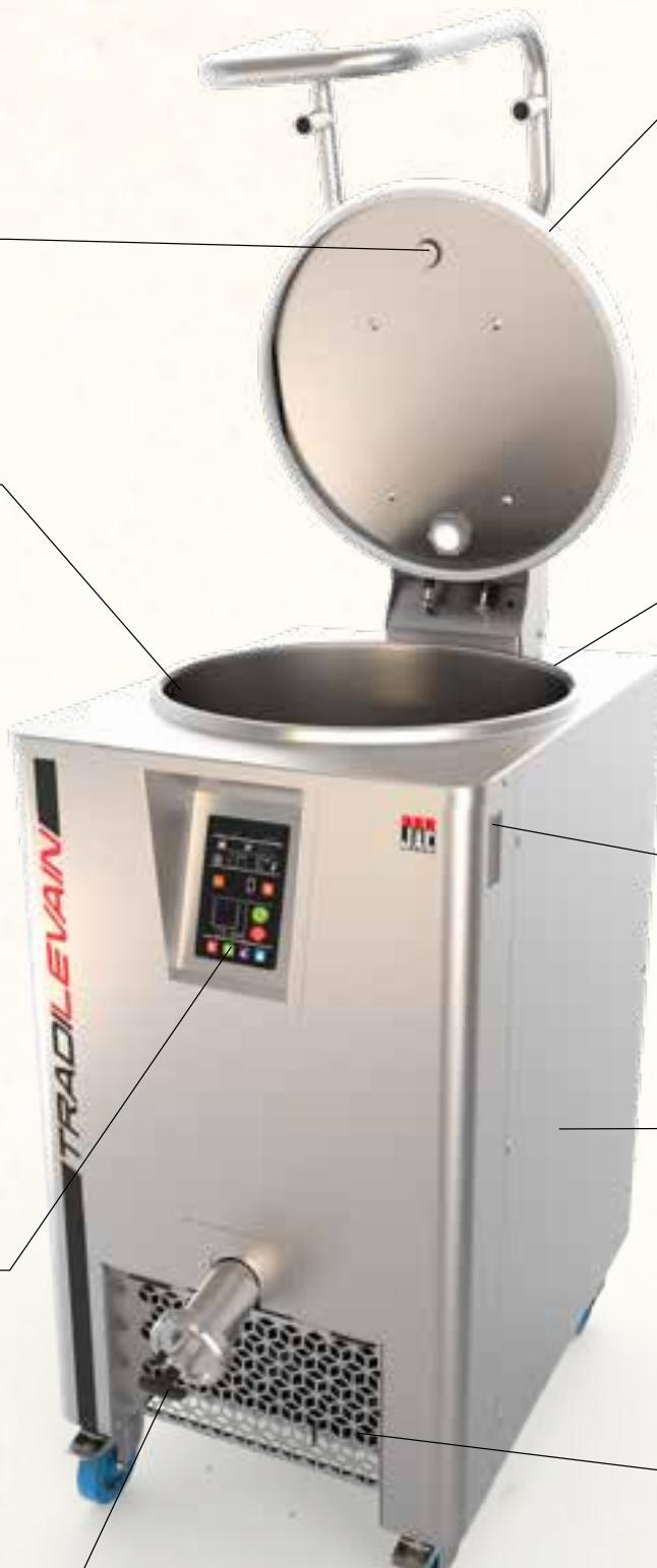
The airtight tank seal is placed around the lid. It can be dismantled in a few seconds for easy cleaning.
