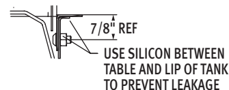
Sectional View Showing Table Connections
