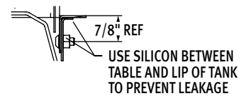
Sectional View Showing Table Connections
