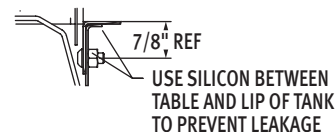
Sectional View Showing Table Connections
