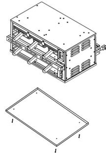
**Step 2** Place bottom unit into position then stack the next unit on top. The top of the lower holding unit rests inside of the base of the upper unit.
