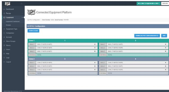
After programming the wells two options are then available. "DOWNLOAD PHU CONFIGURATION FILE" will create a local RCP formatted file with the programming. Alternatively, the "SAVE button" can be selected. This will update the well programming on the unit instantly from the DCEP to the RFHU unit itself. This is a real-time recipe program update.
