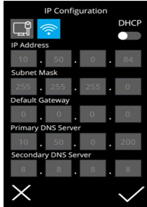
Selecting on any of the 5 Network Settings will load an on-screen numeric keypad where the IP address details can be entered manually.
