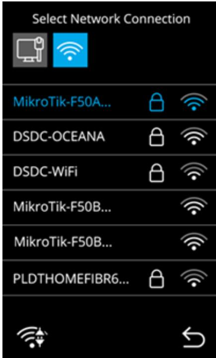
To disconnect from the WiFi select the disconnect icon (📶) in the lower left hand corner of the RFHU or alternatively click on another WiFi SSID to join a different WiFi network (WiFi password entry will then be required).
