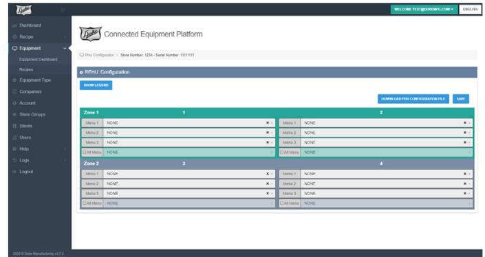
The RFHU programming grid will be color coded per zone. Recipes programmed within each zone will be required to be of the same top temperature and bottom temperature.
