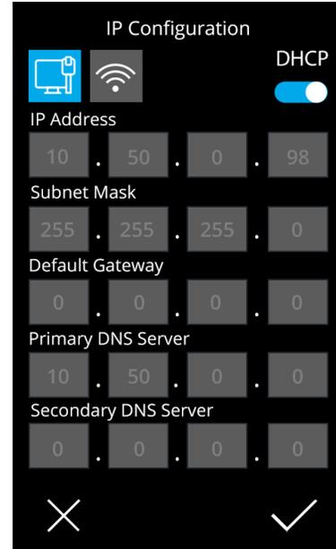
Network Config can be set to “Read Only” mode if the access is locked within Tools menu. Alternatively, if “Network” is unlocked in the Access menu then changes can be made to the selected network.
