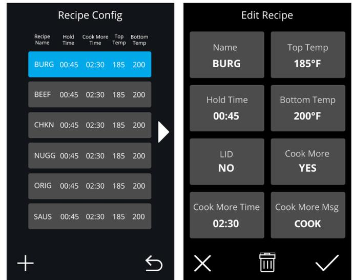
Key information on each recipe is displayed on this screen view. This includes the Recipe Name (appears on the well on the runtime screen), the Hold Time, Cook More Time, Top temperature and the Bottom Temperature.
