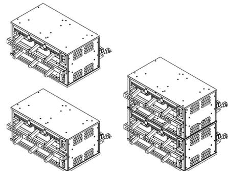
**⚠ WARNING** TIP HAZARD! DO NOT STACK RFHU-42 OR RFHU-34 UNITS. DO NOT EXCEED 2 HOLDING UNITS PER STACK. DO NOT PLACE HOLDING UNIT STACKS ON SURFACES THAT MAY EASILY TIP OVER.
