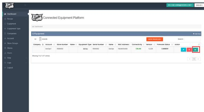
After selecting the "Dashboard" icon to connect to a specific RFHU the programming grid will appear. As this is a connected unit the unit configuration will be detected automatically, for example a 2x2 RFHU configuration appears below.
