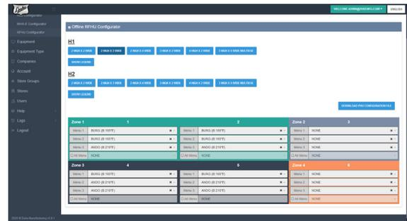
When finished select "DOWNLOAD PHU CONFIGURATION FILE" option. This will create a RFHU "RCP" file which contains both the recipe list and well mapping settings.
