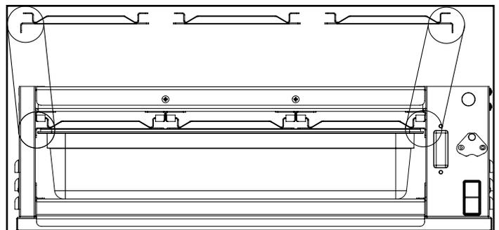
These are just a few of the multiple pan options possible that you can configure without the use of tools and with the standard parts included with your unit.
