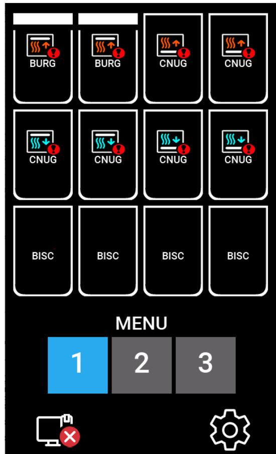
1. Top Heater High Temperature Fault
