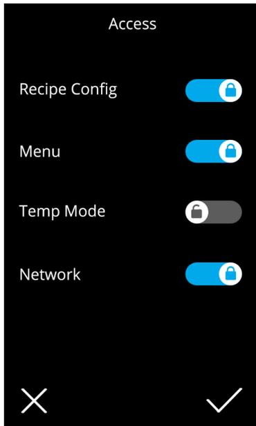
Each of the Recipe Config, Menu, Temp Mode (C/F) and Network can be locked or unlocked.
