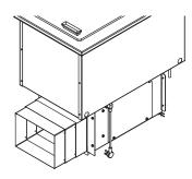
5. Put eight provided screws through the telescoping duct side walls to hold it at the desired depth.
