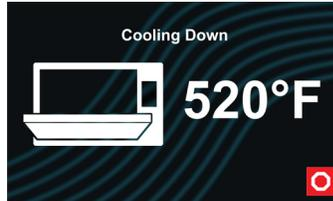
"Cooling Down" screen appears and stays on until oven temperature is below 200°F (95°C)
